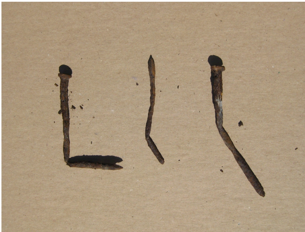
#2. Corroded Deck 2 nails
