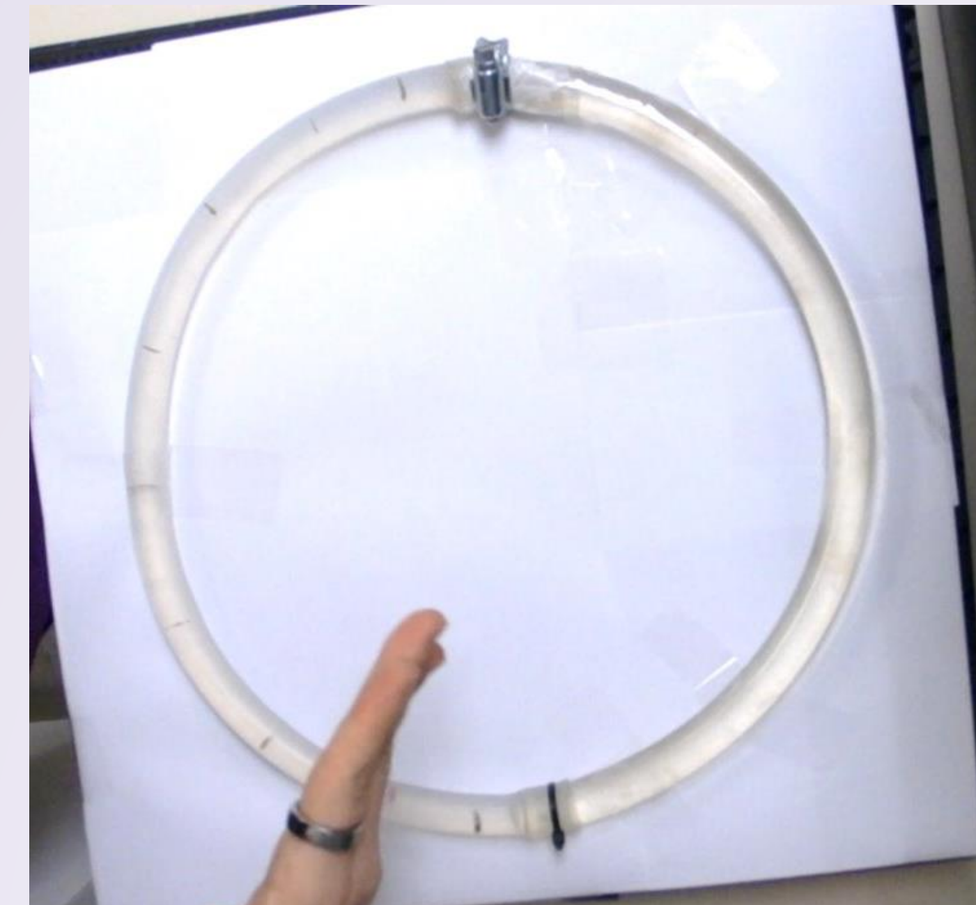
Above: First iteration of our test setup. Two 1/2" inner diameter Tygon tubes, one more rigid and one flexible, are joined in an 11" diameter loop. Compressions are applied manually by hand as pictured.
