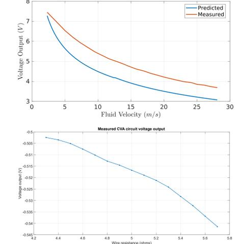
Fig. 2. Top and bottom show figures CCA and CVA operation respectively. Both are calibration curves that can be used to estimate wind speed or wire resistance from voltage measurements.
