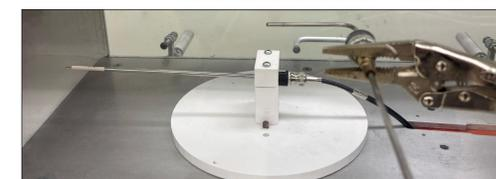
Fig. 3. Hot wire in a wind tunnel for collecting experimental data. Research was done to understand each of the
