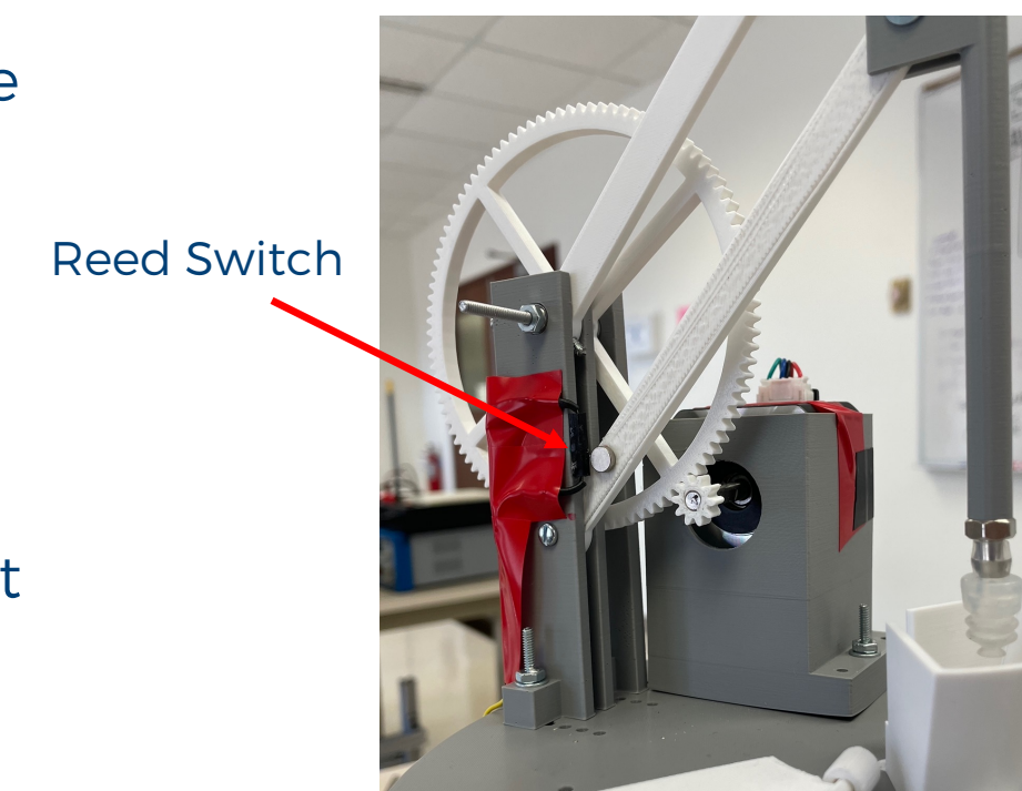
Pickup arm with reed switch
