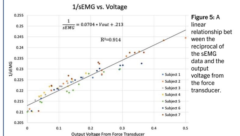
Figure 5: A linear relationship between the reciprocal of the sEMG data and the output voltage from the force transducer.
