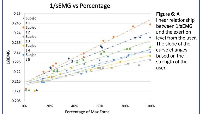
Figure 6: A linear relationship between 1/sEMG and the exertion level from the user. The slope of the curve changes based on the strength of the user.
