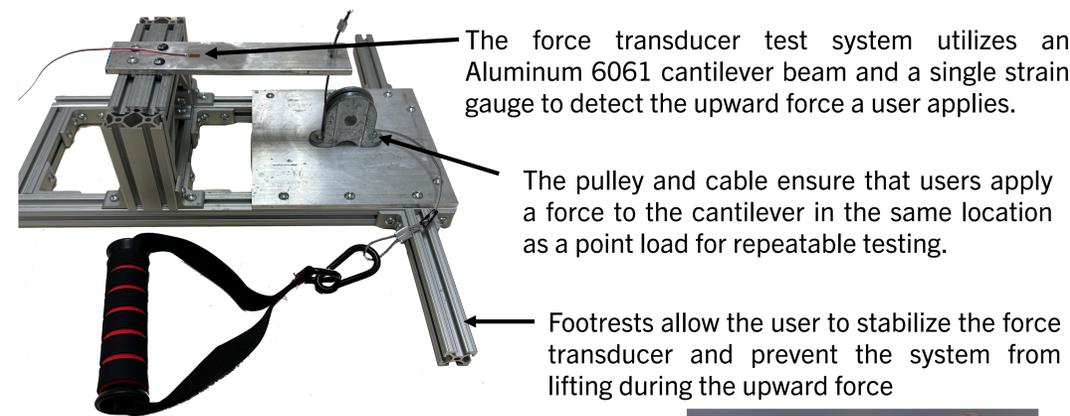
Figure 3: Finalized Force Transducer Test Fixture
