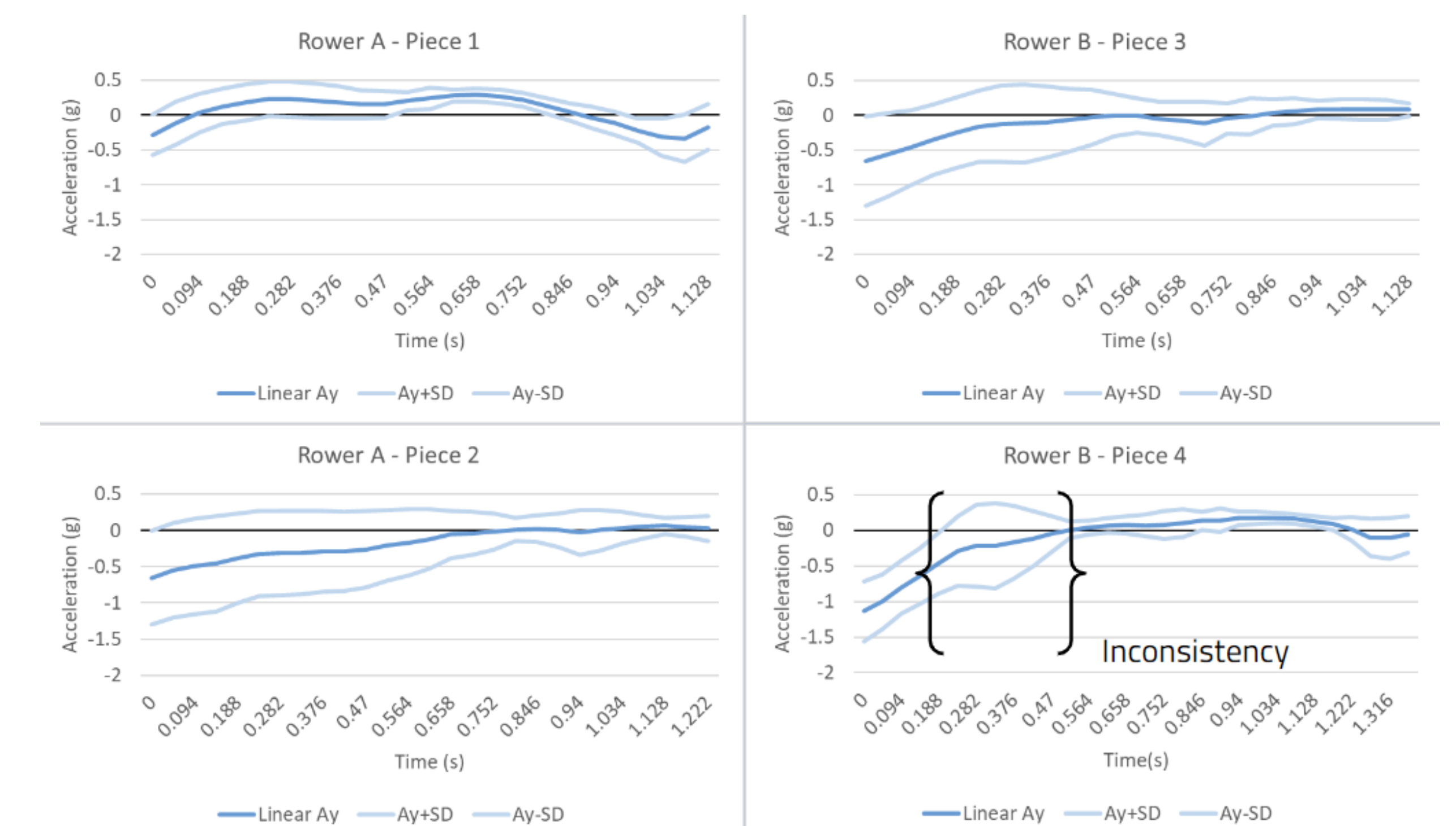
Figure 6: Four sets of phase averages from two female rowers from on-water trials. Note that Rower B is generally a more consistent rower due to a smaller standard deviation, while Rower A produces slightly more power to overcome the drag forces of the boat.
