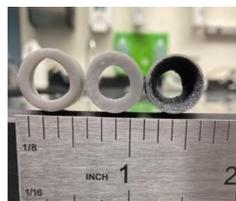
3D printed valves; smooth case with two different restriction severities on the left, added roughness shown on right
