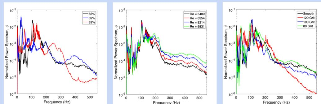
Normalized Power Spectrum For A Fixed Re = 5407, In A Smooth Case For Different Restrictions
