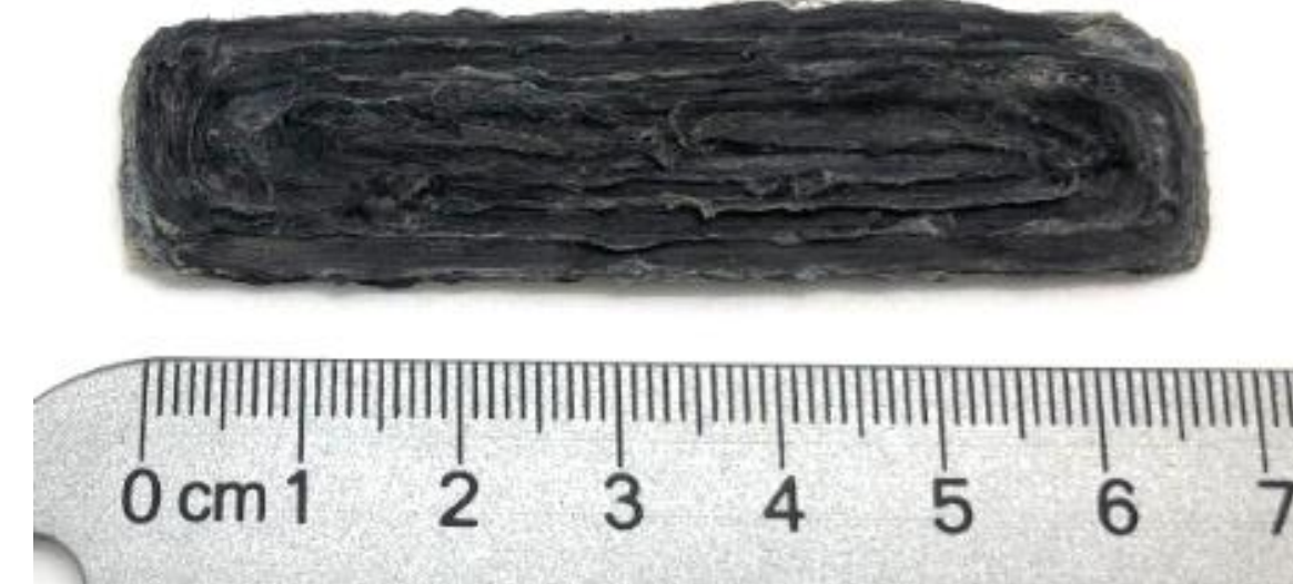
Figure 3: Final print result of warp-specimen sample geometry
