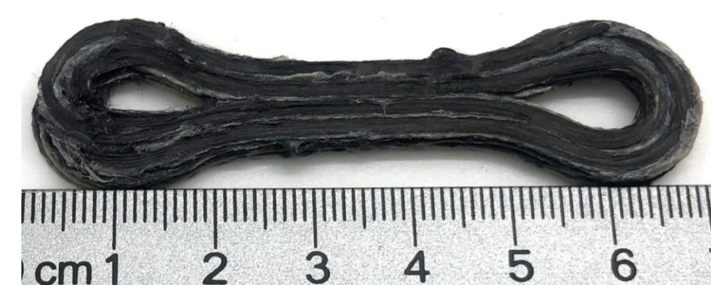
Figure 5: Final print results of barbell sample specimen geometry
