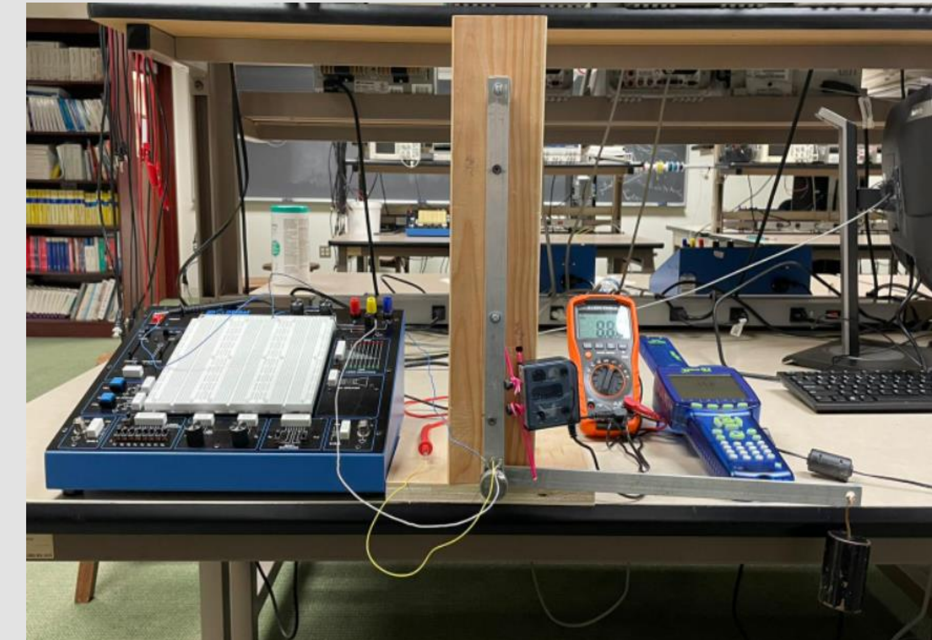
Figure 2: A prototype of an arm.. Force transducer was used to measure the bicep forces.
