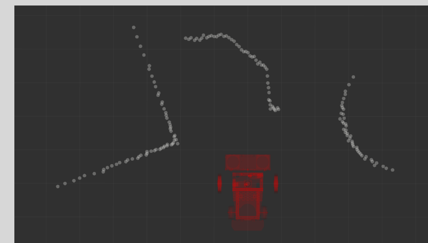
LiDAR scan containing the dock along with environmental obstacles
