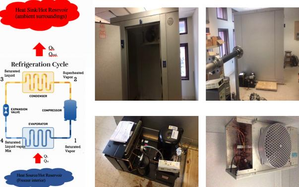
Figure 1 (Left) : Vapor is condensed to liquid in the condenser, thus giving off heat at a high temperature to the surrounding environment. Finally, the high pressure, high temperature liquid leaving the condenser is cooled and reduced in pressure by passing it through an expansion valve.
