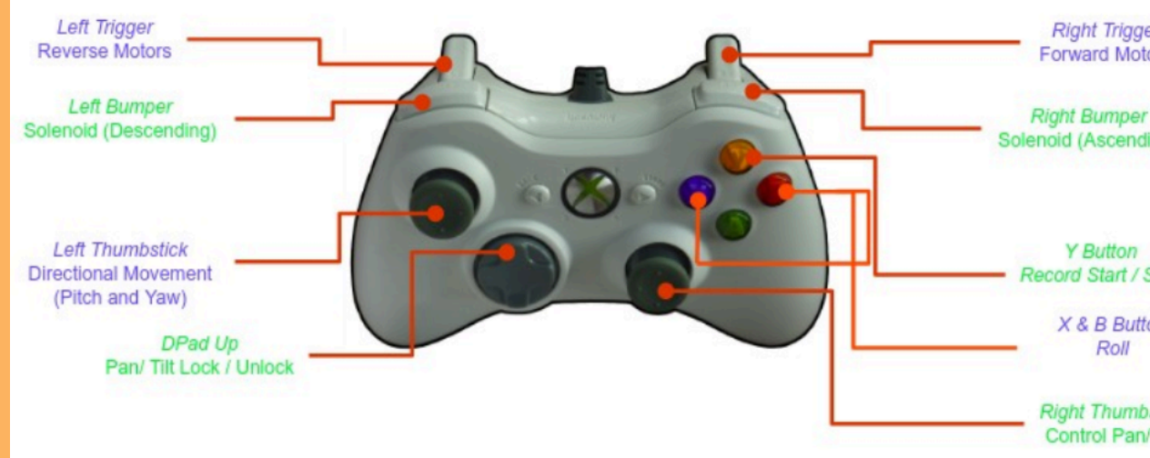
Figure 4. R.O.V controller layout, using Xbox 360 remote
