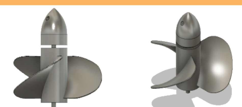
Figure 2. CAD model of the propellers designed for the Hobbyking ST3508 motors
