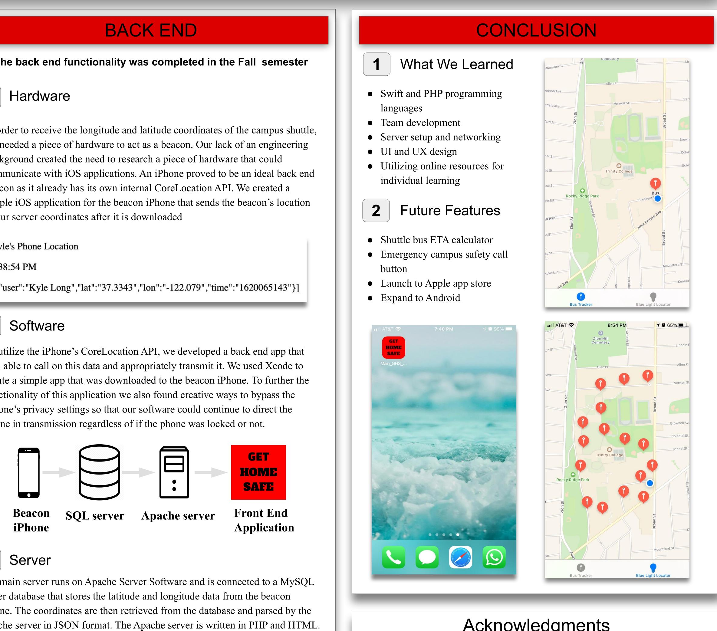
The Get Home Safe app connects to the server and reads coordinate updates in real time. These coordinates are then used to update the bus marker so that users can watch the bus icon move as the bus moves.
