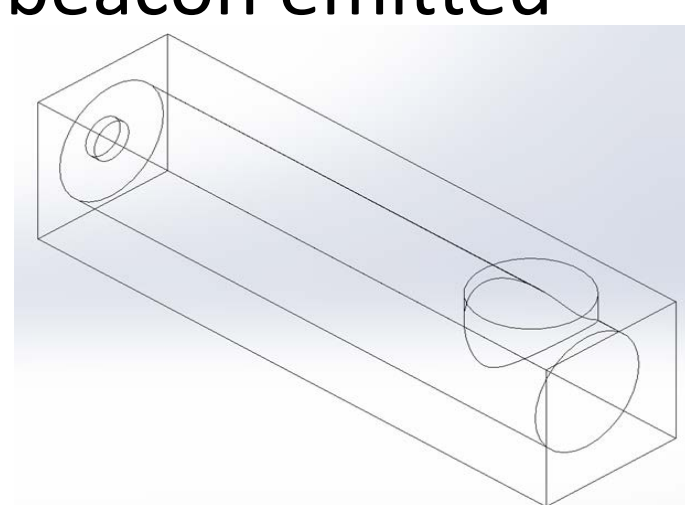
Figure 6: 3D print design to host IR Diode
