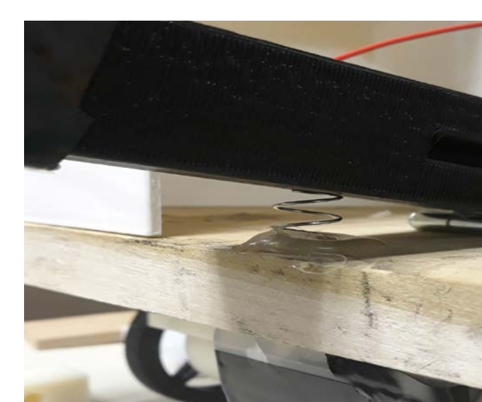
Figure 11: Spring applying upwards force to allow mechanisms to lock
