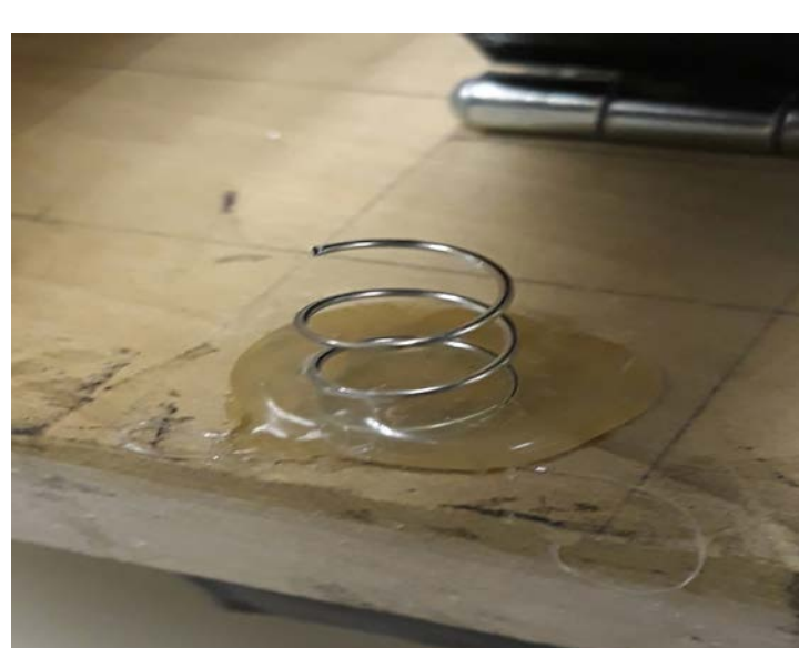
Figure 10: Spring held in place by glue from a glue gun
