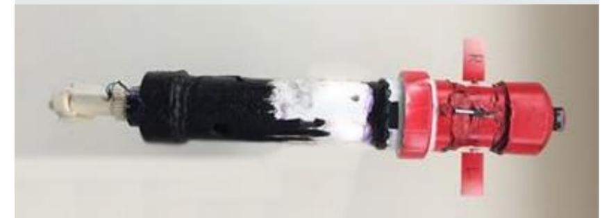
In its current state, the biomimetic AUV may serve as a platform for additional features including advanced water sampling, such as pH measurement, or underwater photography.
