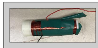
Figure 2: Inductor Coil
