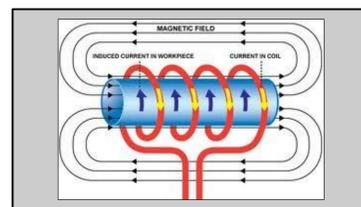
Figure 1: Electromagnetic Induction Theory [1]
