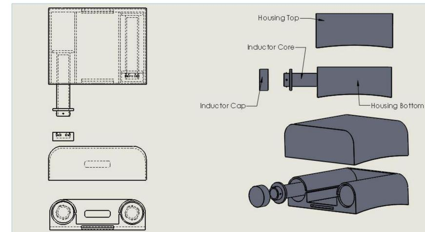
This housing system was 3D printed using ABS plastic for its low magnetic permeability and lightweight. The housing consists of a top piece and a bottom piece. The bottom holds the two inductor components, the circuitry, and the battery, while the top piece is secured with Nylon screws to contain the entire assembly. The housing is contoured on the bottom to fit better on the wearer's leg.
