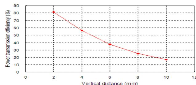
Graph 1: Measured Outcome from literature of Vertical Distance vs Power Transmission Efficiency [1]
