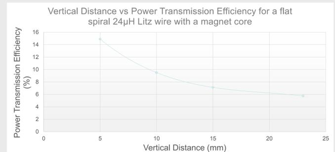
Graph 2: Vertical Distance vs Power Transmission Efficiency for the flat spiral 24µH Litz wire with a ferrite core
