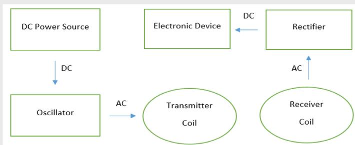
Figure 1: Wireless Charging Device Block Diagram
