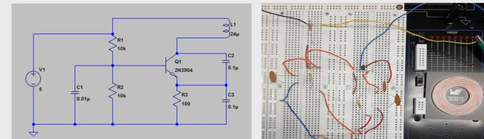
Figure 2: Schematic and Experimental Setup of the Transmitter Circuit
