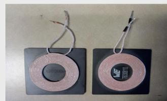
Figure 4: Litz wire 24µH flat spiral coils with a magnet core
