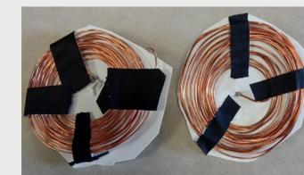
Figure 7: Hand-build copper 2.2µH flat spiral coils
