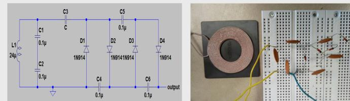
Figure 3: Schematic and Experimental Setup of the Receiver Circuit
