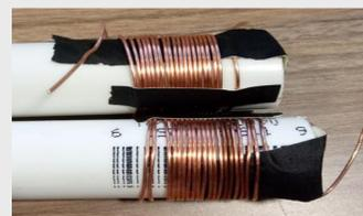
Figure 6: Hand-build copper 2µH cylindrical coils
