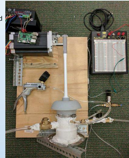
Figure 3: Pulsatile Pump Design
