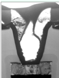
TEM image of IC chip interconnect.
