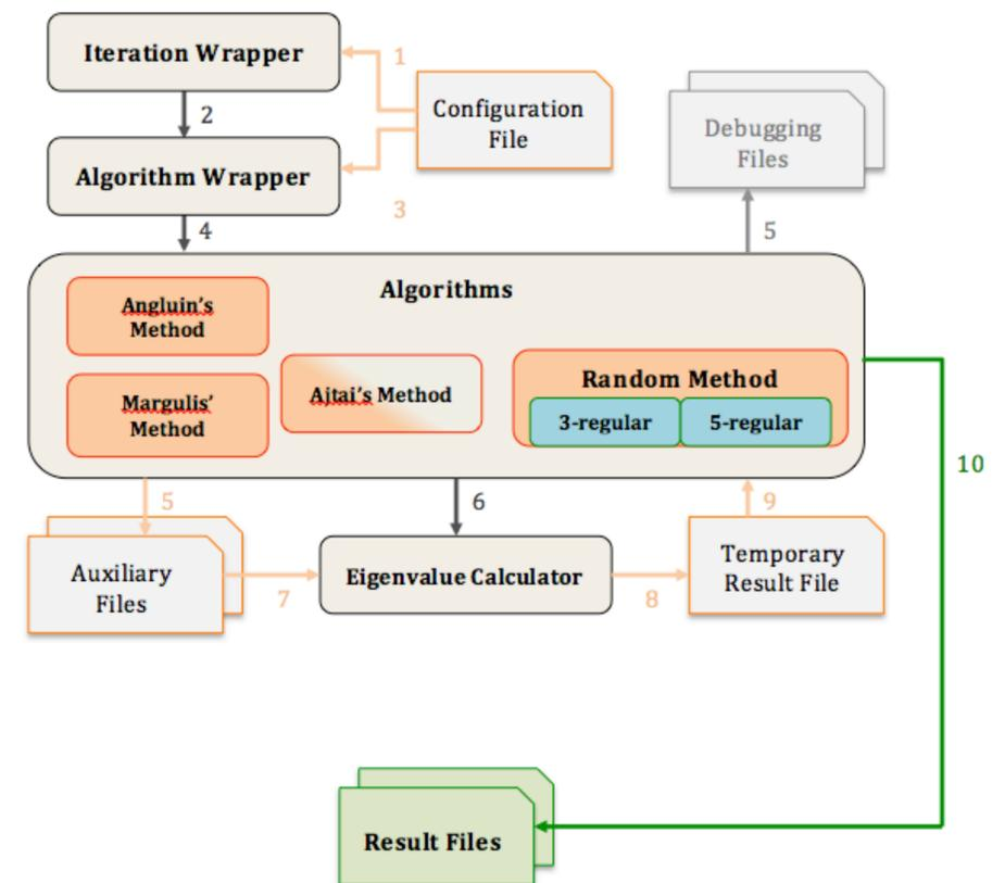
(Fig. 4) Program execution flow of the expander package
